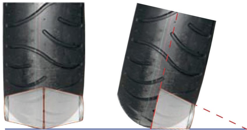
The rolling circumference decreases: The front fork geometry and the rounded profile of the tyre makes the bike turn automatically when leaned over.
